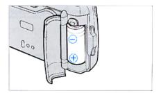
Insert the battery as indicated on the inside of the battery chamber, then snap the cover shut.
